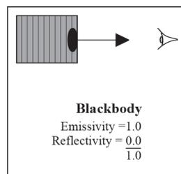
Shiny metal surfaces act like mirrors, with emissivities in the range 0.05 to 0.2. Accordingly, they have only 4% to 25% emitting area compared to reflecting area, and for that reason are difficult to measure with infrared methods. Non-metals, organic materials, and coated metals have emissivities in the range of 0.8 to 0.95 and thus have 400% to 1900% emitting area compared to reflecting area, and thus are much more easily measured successfully.
