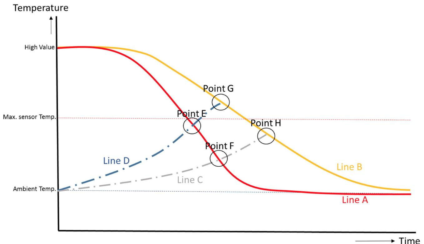
During operation a curing system will “store” a lot of energy in the unit, shown in the graph as the “High Value”. The Max. sensor temp is the maximum temperature the sensor can handle before permanently breaking down (max 212°F for standard IRT/c’s). The Ambient temperature is the temperature of the air that is moved through the system by the ventilator.
