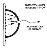
"You see, Alice, the shiny, reflective cup on the D-series does the same thing that you saw in your mirror. Instead of your eyes, a sensitive detector is used to look into the hole.
