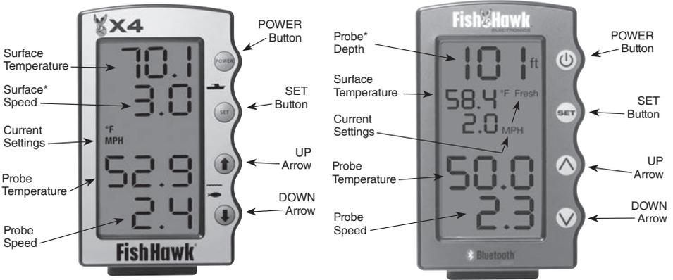
The POWER button turns the display on and off. The display draws 35 mA when on and .3 mA when off. The display is equipped with a backlight for low-light conditions. Enable the backlight by pressing the UP arrow or turn the backlight off by pressing the DOWN arrow. The model X4D has three levels of backlighting.
