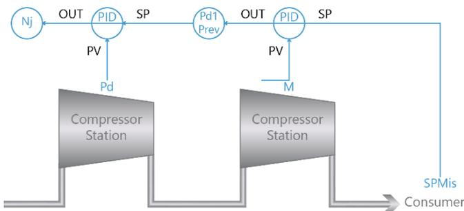
**Figure 4 – Controlling compressor stations and compressors**
