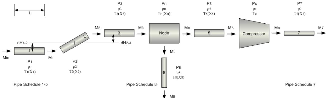
Figure 1 – Dividing a pipeline into segments
