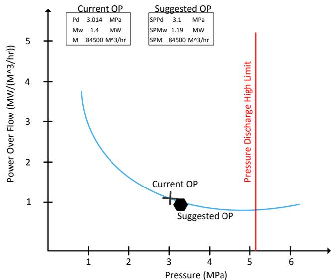
**Figure 11 – Power over flow curve for Compressor Station 1**
