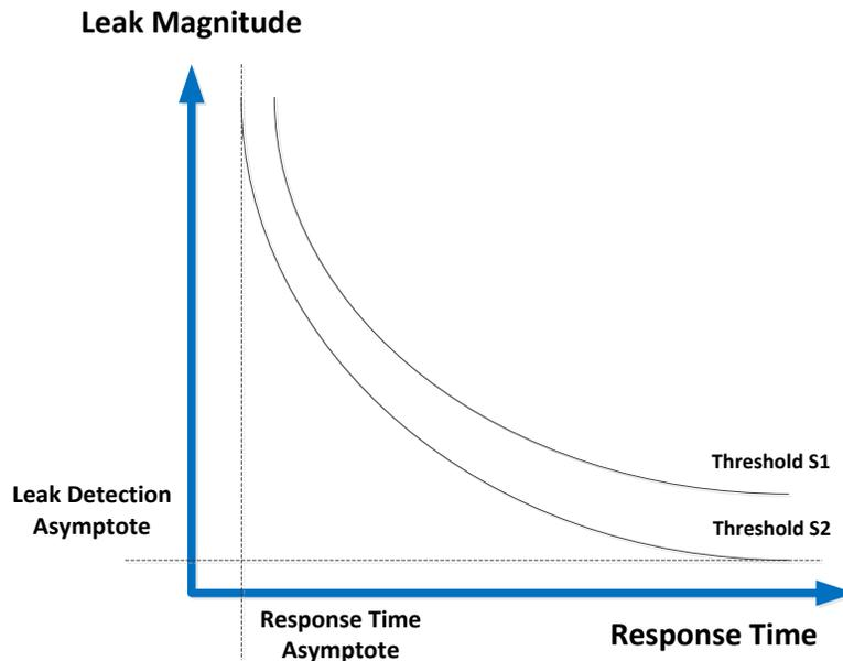
Figure 1. *OptiRamp* LDM sensitivity curves
