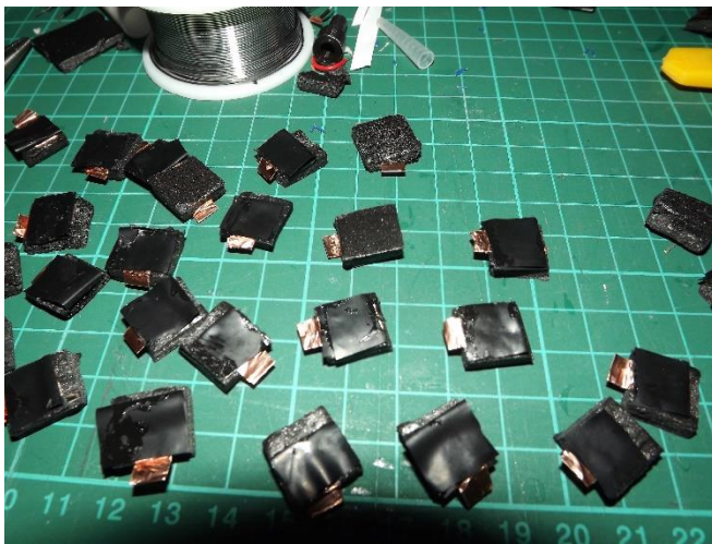
Figure 5: FSR sensors, second stage (Velostat application)
