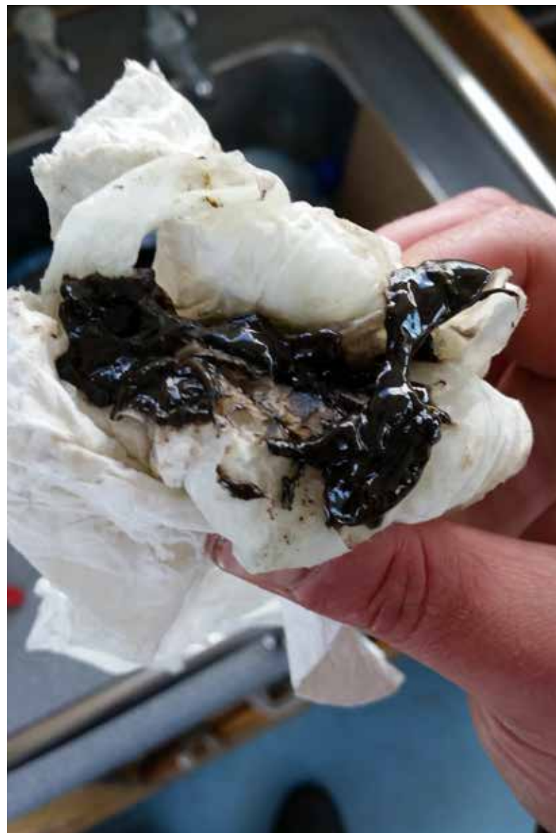
▲ Asphaltenes are identifiable as a black, shiny, tar-like substance which settles on the bottom of the fuel tank.
