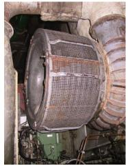
Yet there is another fuel saver, right under everyone's nose, it's not sexy or cutting edge, it's not the latest innovative technology and is used on all high speed engines - the air filter on the turbocharger.
