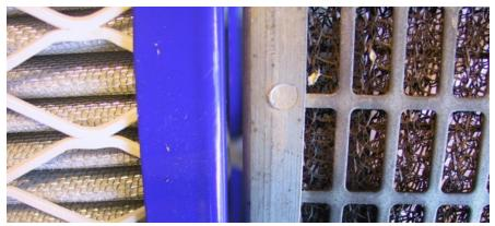
Of course many engineers acknowledge the problem and cover the air filter silencer with a filter cloth, better than nothing one would assume, but it can actually make the situation worse. Why? The filter cloth quickly gets dirty and as it is the same surface area as the original mesh then it effectively starts to restrict air flow just like any blocked cooler but worse still they are not very effective as the cooler still gets dirty, so the engine now has two restrictions to air flow.
