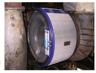
the Caterpillar and Cummins owners don't clean charge air coolers because they have a filter and maintain the SFC.
