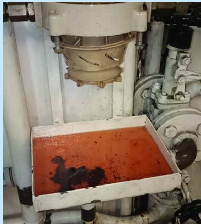
▲ Diesel bug is a growing problem in vessel engines because of changes to fuel composition.
