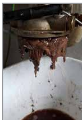
THE PROBLEM: An example of diesel bug
