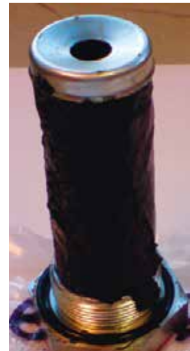
Left, right and far right: Fatty acid methyl ester (FAME) that's found in conventionally produced biodiesel can leave a waxy residue on filters
