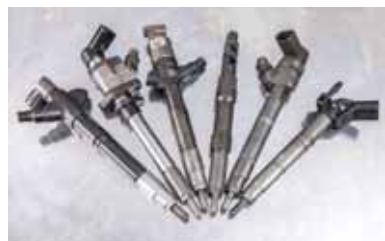
Modern injectors can open and close 100 times a second, so fuel quality is paramount.
