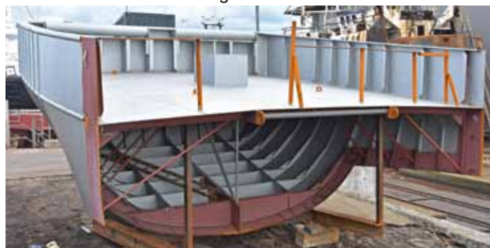
... for which a new transom section is ready to place in position.
